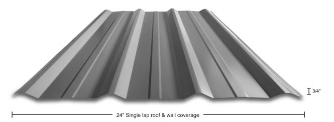
Deep-ribbed for strength, Hi-Rib Panel is a tailored, modern look for buildings, sheds or patio covers. 3/4" high rib 8" on center. 26" wide with 24" coverage. Hi-Rib is a narrow panel, making it much easier to install.
